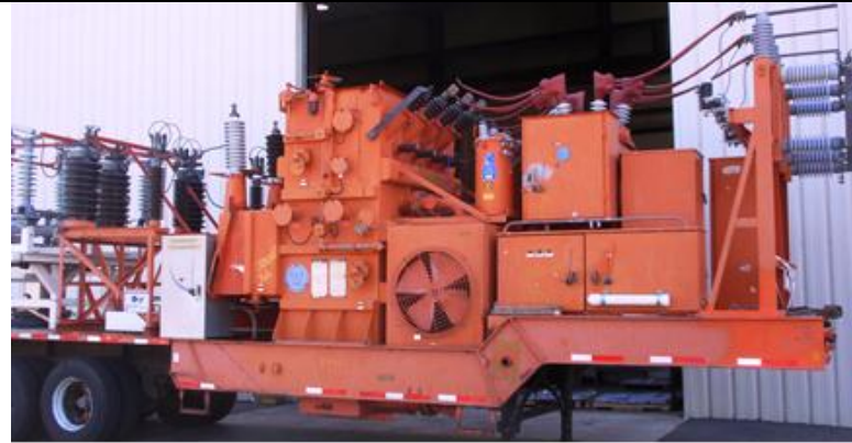
9 MVA 69 x 34.5 - 4.36Y x 13.8Y Westinghouse
