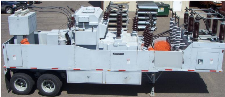
5 MVA 69Y - 34.4 x 13.8 x 12.47Y – 7.2/12.47Y x 2.4/4.16Y Westinghouse
