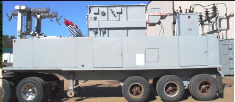
10 MVA 69 - 12.47Y x 24.94Y Westinghouse
