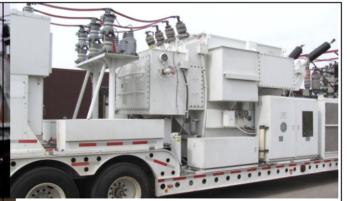
20 MVA 69 x 43.8 - 12.47Y x 24.94Y Delta Star w/ LTC
