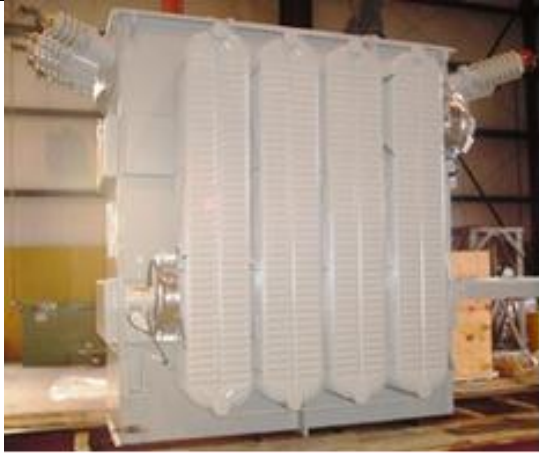
5 MVA 46 x 22.9 - 24.9Y x 12.47Y Kuhlman
