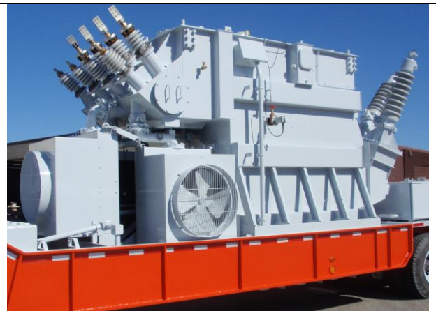
20 MVA 115 - 24.94Y x 13.2Y x 2.4/4.16Y/2.4 Westinghouse
