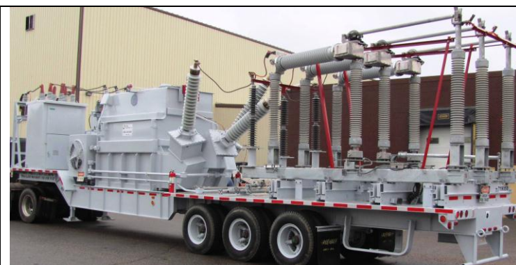
10 MVA 161 - 13.8Y Westinghouse
