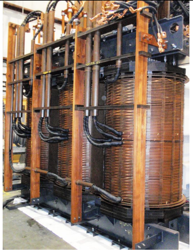
Partially distributed RV or taps windings
