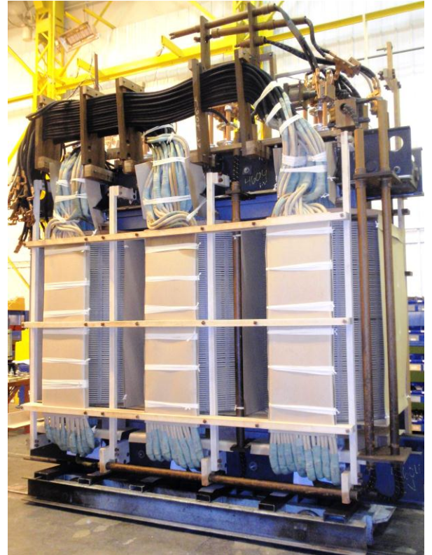
Short circuit strength is greatly improved and braised joints are eliminated in the windings
