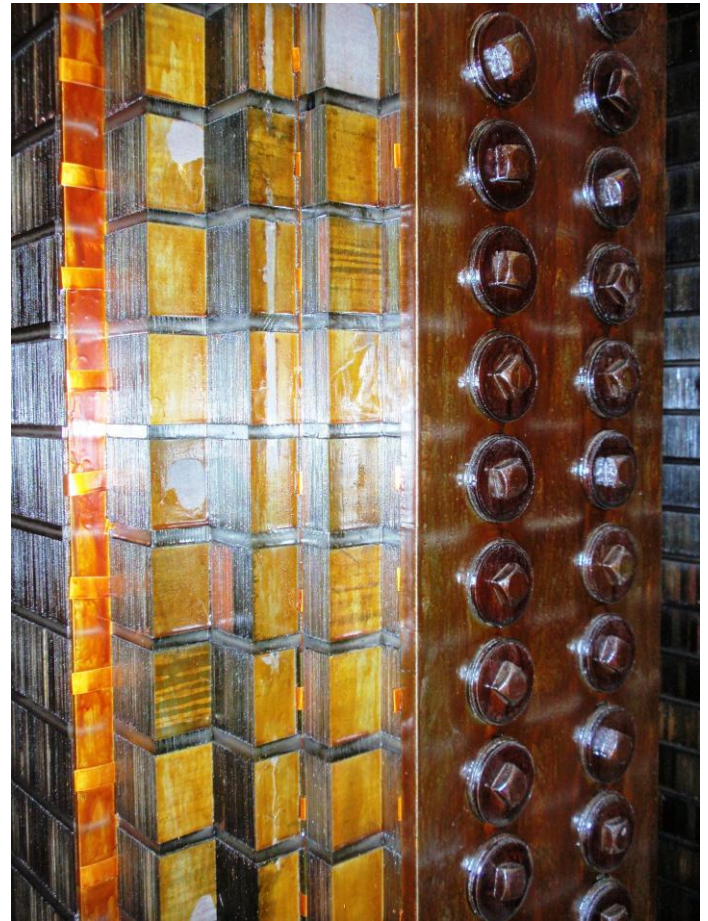
Original Reactor Core with Gaps
