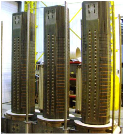
New Assembled Core with Gaps
