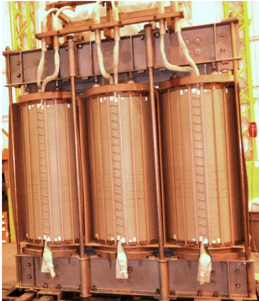
Fully Assembled New Core & Coils
