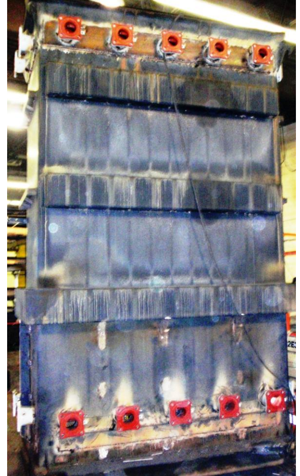
Installation of new flanges
