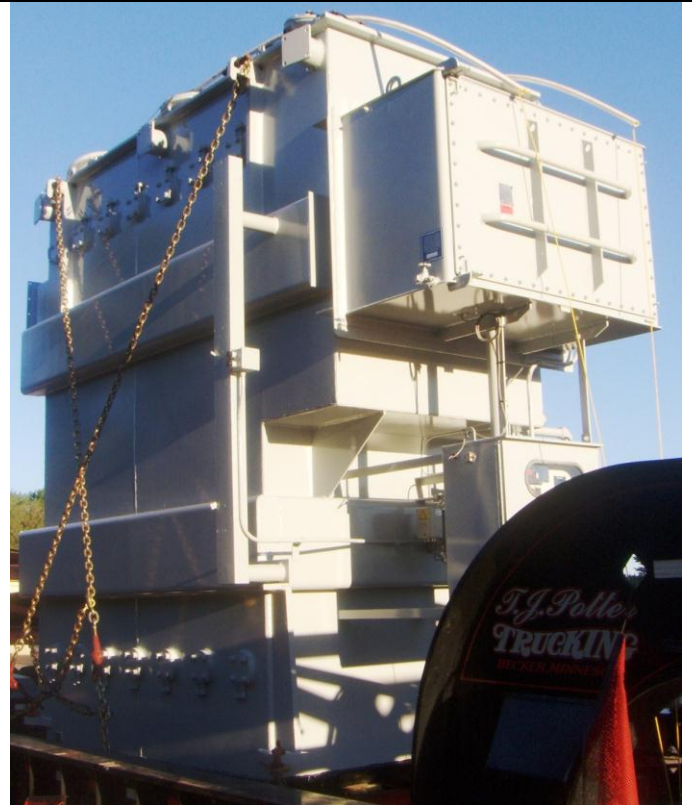
New Reinhausen RMV-II & Control Cabinet
