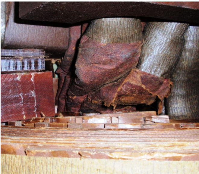
Gassing Due to “Telescoping” of LV Windings
